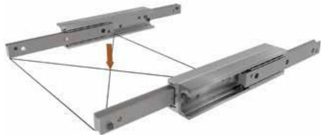
Ideal mounting configuration with two parallel NTSG, load in preferential direction applied in the middle of the sliders.
