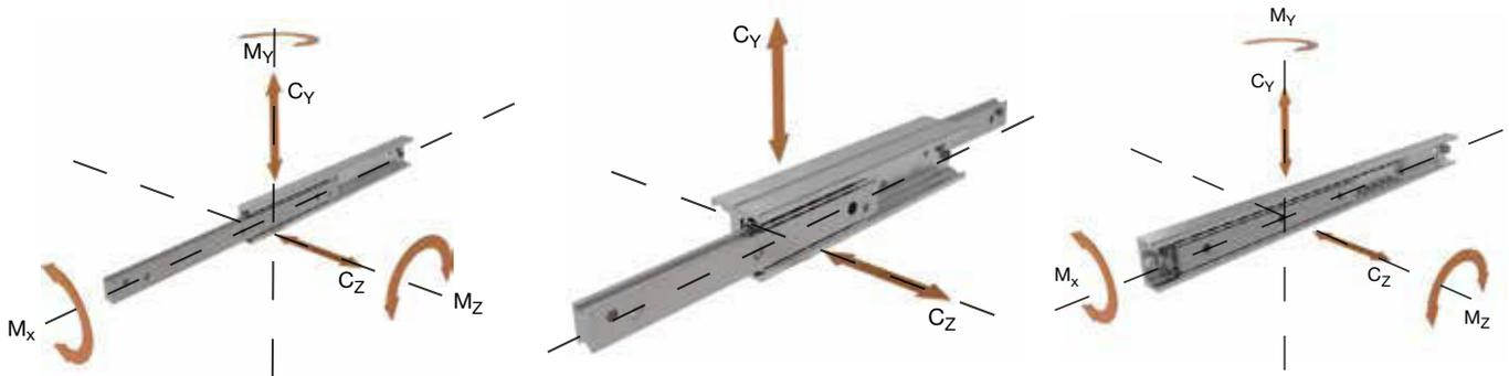
Load capacities are expressed in N (Newton), torque load capacities are expressed in Nm, refer to the Cartesian axes with origin in the centre of the slider and are valued according to standard ISO 14728-2. Tables of load capacities in the following pages refer to a single slider and are to be intended as maximum static admissible loads for a smooth operation.
